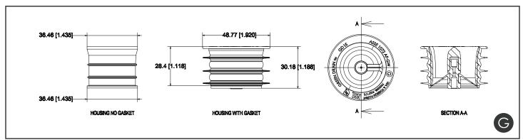
**Specification:** Green Drain (model: GD2) Waterless Trap Seal for 2" Drains. ABS Plastic Housing | One-way Silicone Valve | Silicone Gasket
