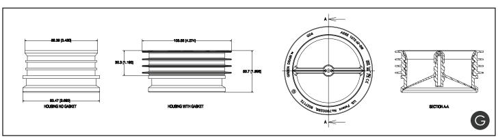
**Specification:** Green Drain (model: GD5) Waterless Trap Seal for 5" Drains. ABS Plastic Housing | One-way Silicone Valve | Silicone Gasket
